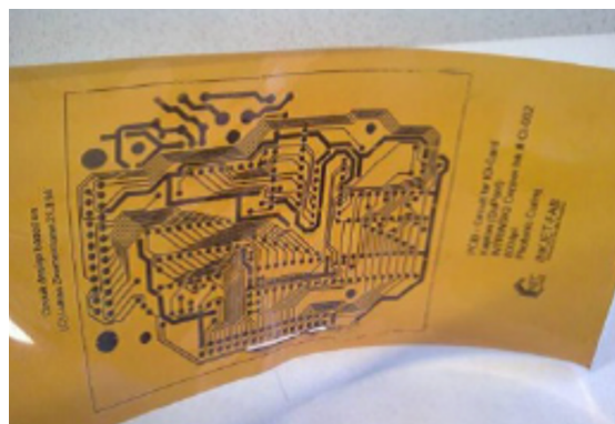
CI-004 printed on polyimide after a reducing formic acid/argon atmosphere processed @250°C 45 minutes.
